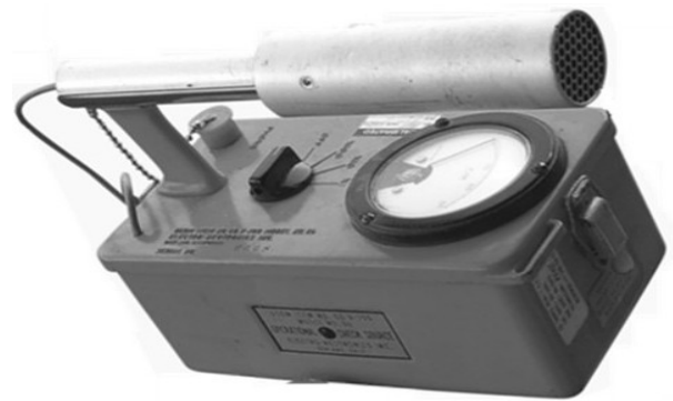
Fig. 3: A typical Geiger-Müller counter setup that can be used for radiation monitoring.
