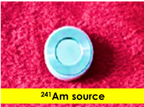
Fig. 2: The ^{241}\text{Am} as alpha emitting source available in the nuclear laboratory.
