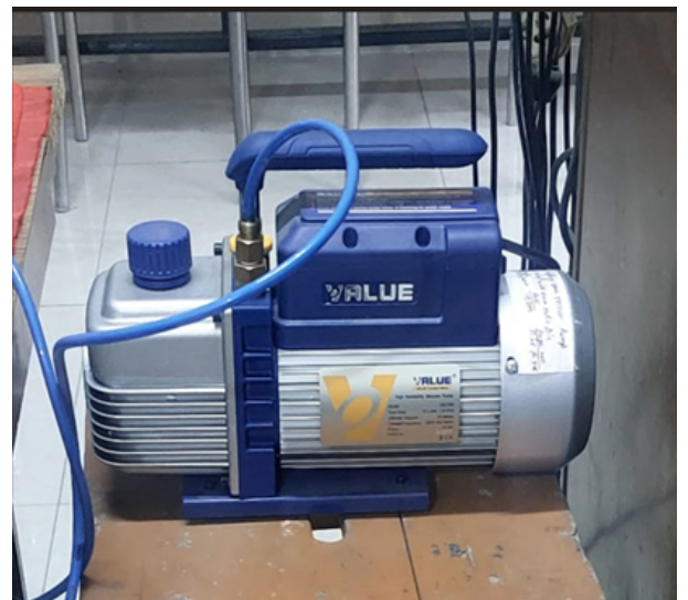
Fig. 3: The Rotary oil pump of “VALUE” make with flow rate 51 Litre/min with \frac{1}{4} HP.
