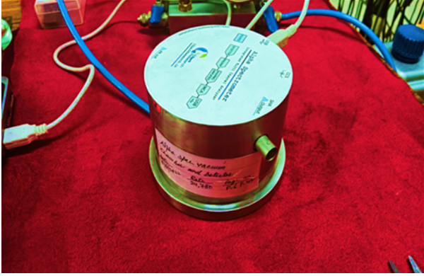
Fig. 1: Vacuum Chamber use in the experiment for determination of thickness.
