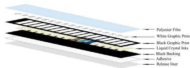
Fig. 7: Schematic diagram of thermochromic LC label construction.
